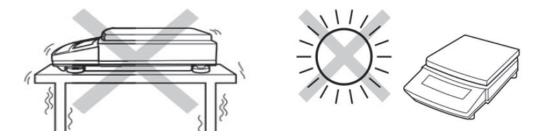
Do not place the scale in locations with excessive temperatures and humidity. For example, directly in front of a heating or cooling vent, a fan, window, or any location with a moving air source. Such a location will subject it to sudden temperature changes, which may result in unstable weight readings.
